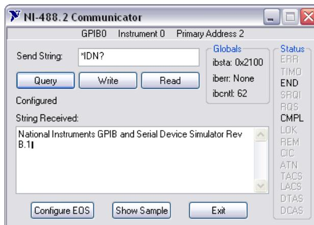
**Figure 5.** Communication with the GPIB Instrument
